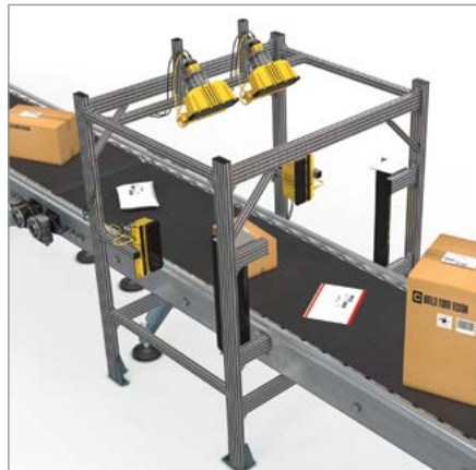
Multi-sided scan tunnel
